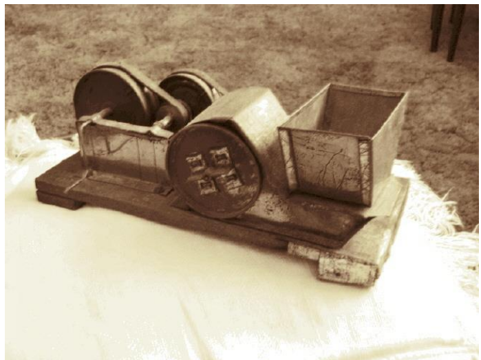
(This blower was forged from tin cans out of the garbage, belt straps of boots, a block of wood, and hob nails out of German boats.)
